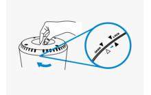
Replace the cover and plug in the air purifier.
