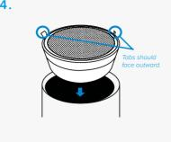
Unwrap the new filters and place them into the housing with the pull tabs facing out.
