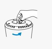
Unplug the air purifier. Flip the air purifier over and remove the filter cover.
