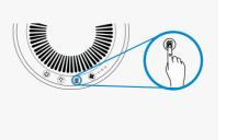
Turn on the air purifier. To reset the Check Filter Indicator, press and hold for 3 seconds. The Check Filter Indicator should turn off.
